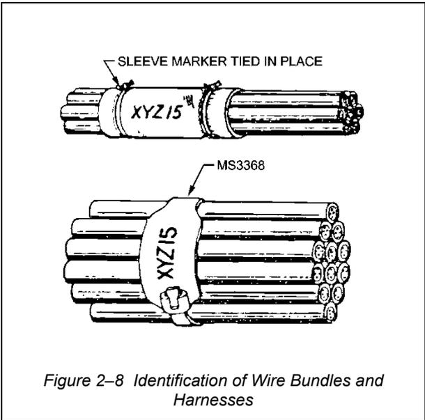
Figure 2-8 Identification of Wire Bundles and Harnesses
