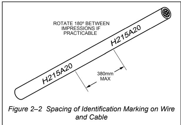
Figure 2-2 Spacing of Identification Marking on Wire and Cable
