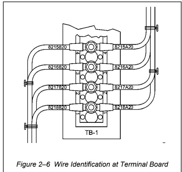
Figure 2-6 Wire Identification at Terminal Board
