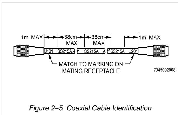
Figure 2-5 Coaxial Cable Identification
